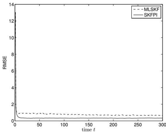
Fig. 2. RMSEs of the considered filters for  $p = 10$ ,  $q = 0.1$ ,  $r = 0.1$ .
