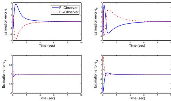
Fig. 1. Estimation error of the P- and PI-Observers without perturbation.
