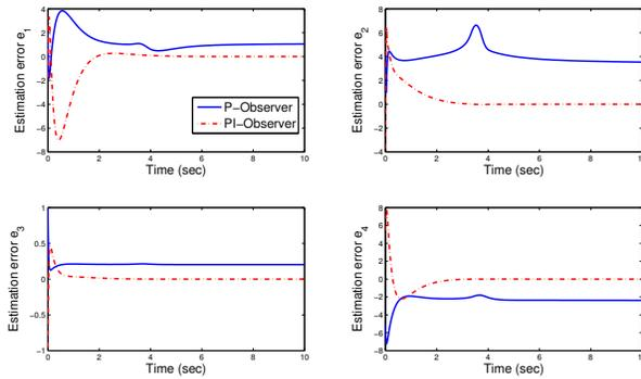
Fig. 2. Estimation error of the P- and PI-Observers with perturbation.
