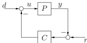
Fig. 1. Standard Feedback Configuration
