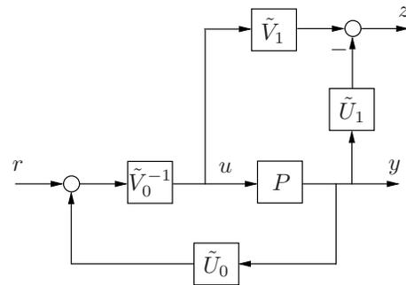
Fig. 2. Experimental setting:  $C_0 = \tilde{V}_0^{-1}\tilde{U}_0$ ,  $C_1 = \tilde{V}_1^{-1}\tilde{U}_1$ .
