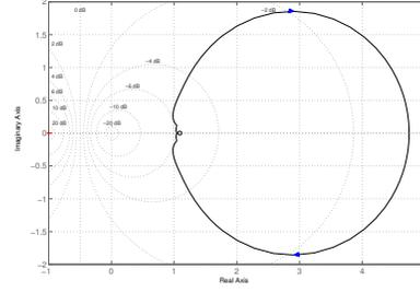
Fig. 5. Nyquist plot of  $T(j\omega)$  in Example 1.
