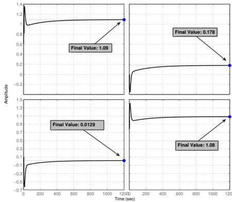
Fig. 6. Step Responses:  $r(t) = \text{step}(t) \cdot e_1$  and  $r(t) = \text{step}(t) \cdot e_2$
