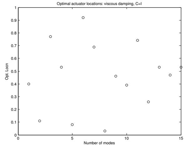
Fig. 1. Optimal actuator location, Viscously damped beam,  $C = I$
