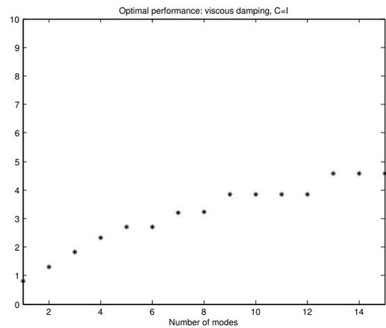
Fig. 2. Performance at optimal location, Viscously damped beam,  $C = I$
