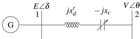
Fig. 1. SMIB system with CSC
