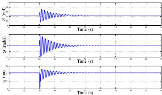
Fig. 6. Closed-loop performance with  $\gamma = 100$  and  $\beta = 40$
