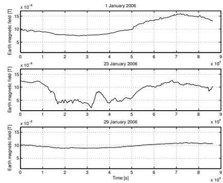
Fig. 3. Time histories of the earth's magnetic field in GEO orbit during three different days of January 2006.
