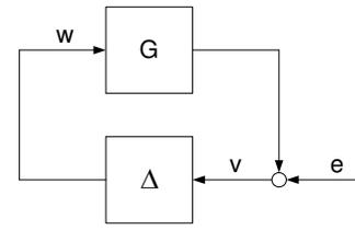
Fig. 7. Model of a system for IQC robust stability analysis.
