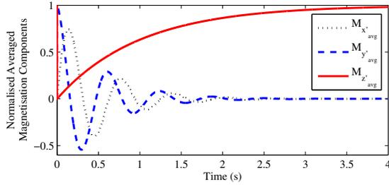
Fig. 2. Approximation for a rectangular pulse excitation through averaging, when  $\Delta\omega = 10\text{rad/s}$ , for a spin system with  $T_1 = 1\text{s}$ , and  $T_2 = 0.5\text{s}$ .
