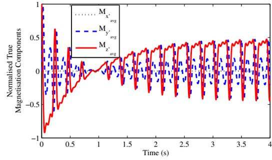
Fig. 8. Exact solution based on simulating the Bloch equation for an on-resonance continuous-wave excitation (31), for the spin system in Fig. 2, when  $\omega_1 = 27\text{rad/s}$ .
