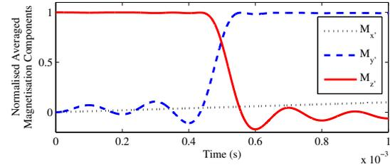
Fig. 6. Averaged result for a sinc pulse during the excitation period, when  $\Delta\omega = 100\text{rad/s}$ , for the spin system in Fig. 2. The pulse duration is  $1\text{ms}$ .
