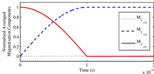
Fig. 4. Averaged result for a rectangular pulse during the excitation period, when  $\Delta\omega = 100\text{rad/s}$ , for the spin system in Fig. 2. The duration of the pulse is  $100\mu\text{s}$ .
