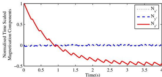
Fig. 11. Evolution of the time scaled magnetisation vector for an on-resonance continuous-wave excitation (31), for the spin system in Fig. 2, when  $\omega_1 = 27\text{rad/s}$ .
