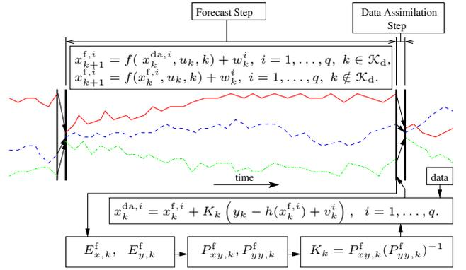
Fig. 1. Diagram of ensemble Kalman filter.
