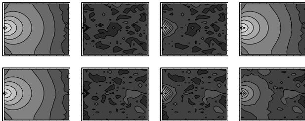
Fig. 5. 2D heat conduction estimation rms error distribution with  $N_d = 6$ ,  $N_s = 1$  (top) and  $N_d = 6$ ,  $N_s = 4$  (bottom). We assume uniform heat conductivity. 1st to 4th columns: rms error distribution of NoDA, Kalman filter, ensemble Kalman filter, and ensemble on-demand Kalman filter, respectively. There is single disturbance to the left boundary edge. Darker regions around measurement points indicate that the errors are reduced by data assimilation relative to NoDA.
