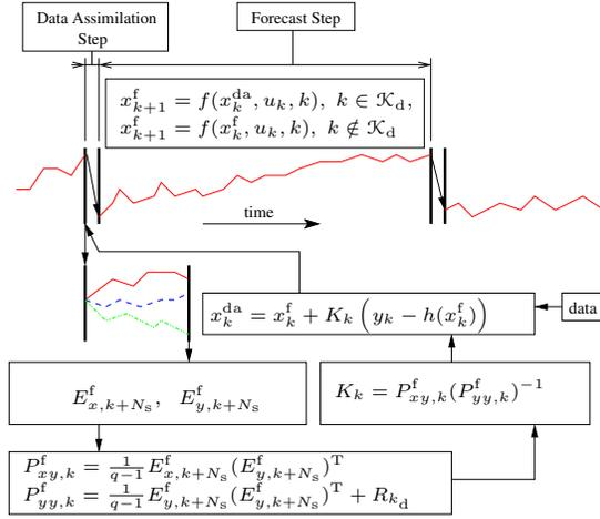
Fig. 2. Diagram of the ensemble-on-demand Kalman filter.
