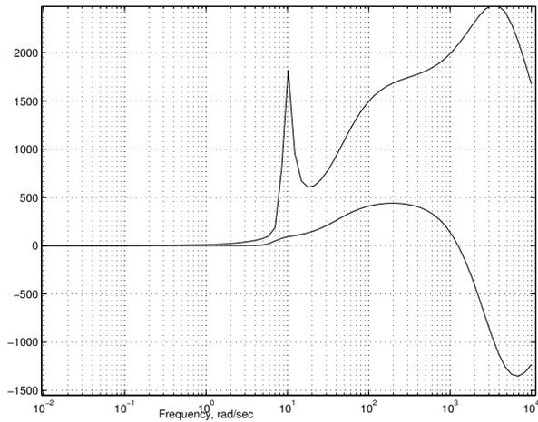
Fig. 2. Eigenvalues of function  $\sigma(j\omega)$  for  $G2$ . Includes the effect of  $R_a$ .
