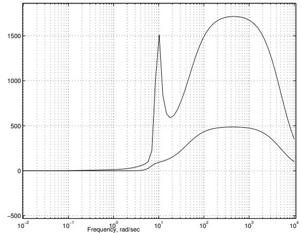
Fig. 1. Eigenvalues of function  $\sigma(j\omega)$  for  $G1$ . No magnetic saturation, no  $R_a$ , constant excitation.
