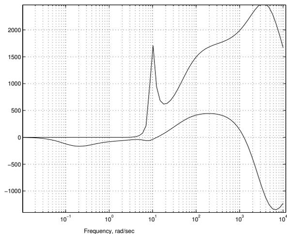
Fig. 3. Eigenvalues of function  $\sigma(j\omega)$  for  $G4$ . Includes the effect of  $R_a$  and excitation control.
