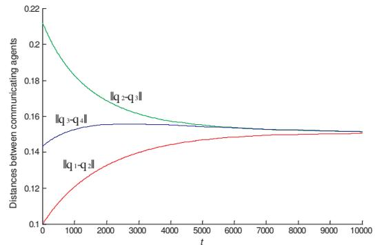
Fig. 1. Four single integrator agents are driven by the control (4) with  $\gamma$  as in (6). The formation graph is a tree. Agents' relative distances are stabilized to the expected desired value  $d = 0.15$ .
