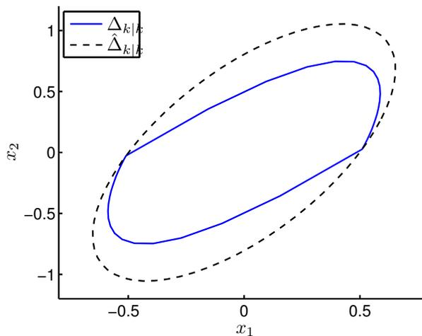
Fig. 4. Actual set bounded error and ellipsoidal approximation used by the Mixed Filter at  $t = 12.9$ , just before an event.
