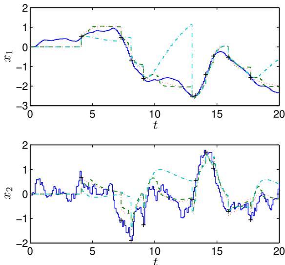
Fig. 2. Actual states and state estimates generated by the observers. Actual states (solid), Mixed Estimator (dashed), Grid Filter (dotted), Kalman Filter (dash-dotted). Events are marked with a + sign.
