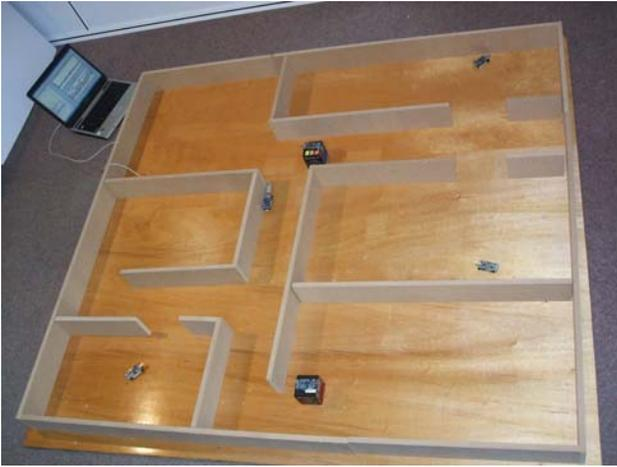
Fig. 5. 802.15.4 Wireless experimental scenario.
