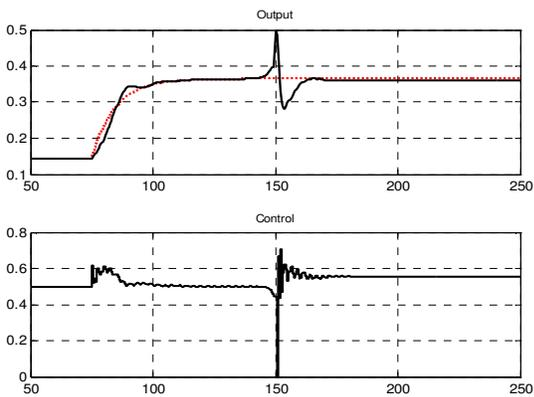
Fig. 7: NGMV output tracking and regulation around an unstable operating point. Upper plot: output (solid), set-point (dotted)
