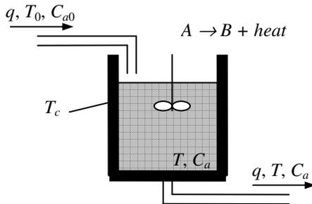
Fig. 5: CSTR Process (input variable is cooling jacket temperature  $T_c$  and output is the concentration  $C_a$ )
