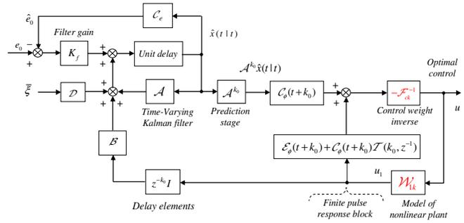
Fig. 4: NGMV Optimal Controller in Kalman Form
