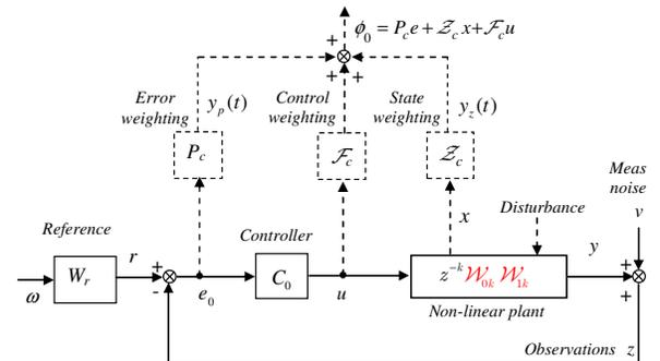
Fig. 2: Single Degree of Freedom Closed-Loop Control System
