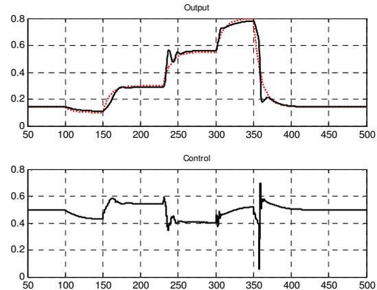
Fig. 8: *NGMV* control: output tracking across the operating range with a gain-scheduled control weighting
