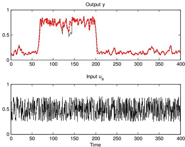
Fig. 6: NARX model validation: plant (solid), model (dashed)
