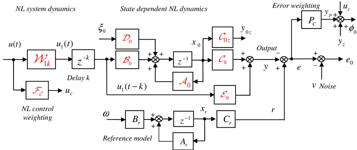
Fig. 1: Nonlinear Unstructured and State-Dependent Plant Model Including Disturbance and Reference
