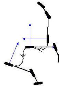
Fig. 6. Admissible trajectory with rapidly changing curvature,  $t \in [25s, 30s)$
