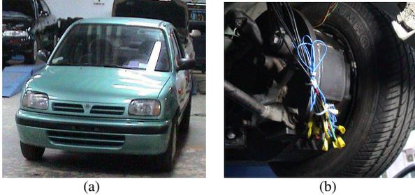
Fig. 1. The experimental vehicle (a) and its wheel motor (b).
