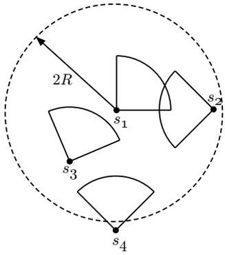
Fig. 3. Neighbor Set of sensor 1. Only the information of the sensors which are in the range  $2R$  from sensor 1 are required to compute the control laws
