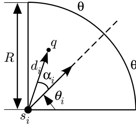
Fig. 1. Limited-range anisotropic sensor model. The sensing performance of sensor  $i$  depends on the distance  $d_i$  and the orientation  $\alpha_i$  from sensor  $i$  to the target  $q$
