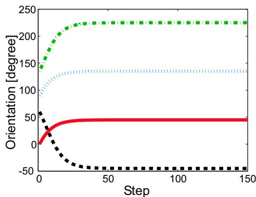
Fig. 8. Evolution of the orientations of the mobile sensors. The mobile sensors are rotating to the center of  $Q$
