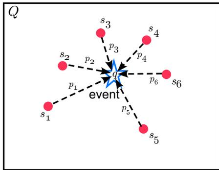
Fig. 2. Joint detection probability. Each point in  $Q$  is sensed by all sensors
