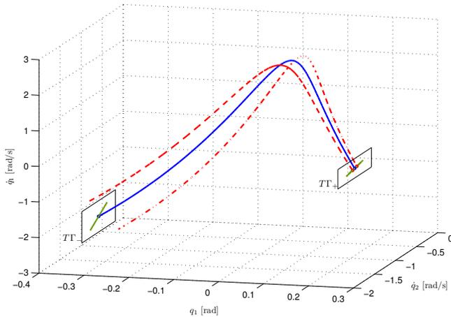
Fig. 5. Desired trajectory (solid) in the subspace  $\{q_1, \dot{q}_1, \dot{q}_2\}$  with continuous-time sub-arc evolving between the hypersurfaces  $\Gamma_+$  and  $\Gamma_-$ . The discrete mapping is invariant, i.e.  $F(\gamma_-) \subset \gamma_+$ . However, trajectories starting on  $\gamma_+$  other than  $[q_*(t), \dot{q}_*(t)]$  do not end up in  $\gamma_-$  (see dashed and dashed-dotted trajectories), i.e. the zero dynamics, defined by the trajectory of the cycle, are not invariant.
