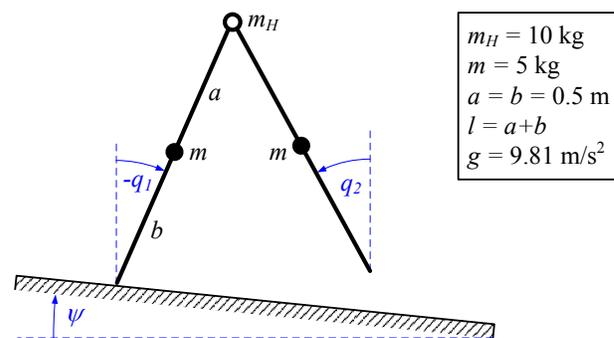
Fig. 1. Schematic of the compass-gait biped on a shallow slope  $\psi$ .
