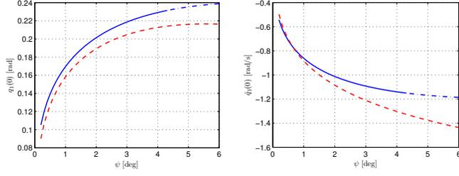
(a) Initial position  $q_{*,1}(0+)$  for the stance leg. (b) Initial velocity  $\dot{q}_{*,1}(0+)$  for the stance leg.
