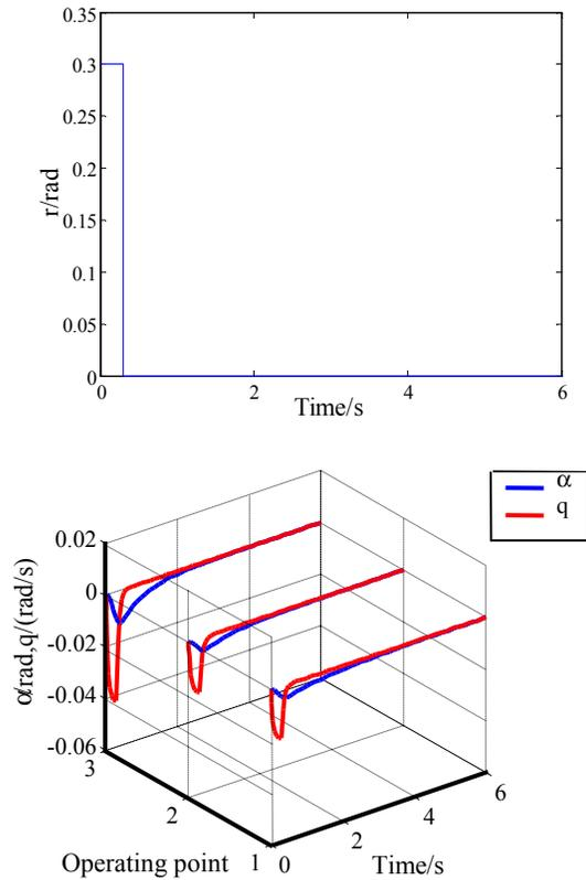
Fig. 1. Response of the airplane on different operating points.
