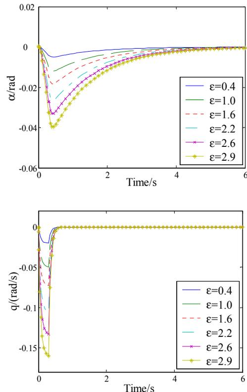
Fig. 2. Response for different  $\epsilon$  on operating point 1.
