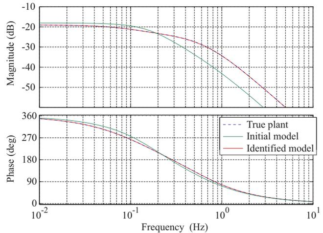
Fig. 4. Bode plots of the true plant, initial model and identified model
