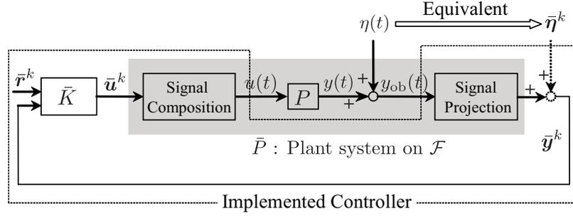
Fig. 1. Block diagram of the control system based on the finite-dimensional signal subspace
