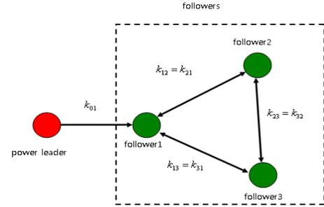
Fig. 5. Coupled network dynamic model containing a power leader and three followers.
