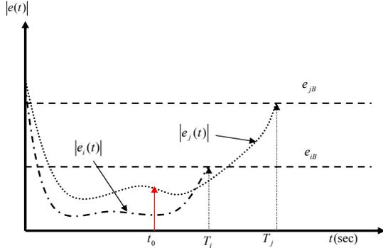
Fig. 4. Fault detection of a power leader using  $i$ -th follower and  $j$ -th follower.
