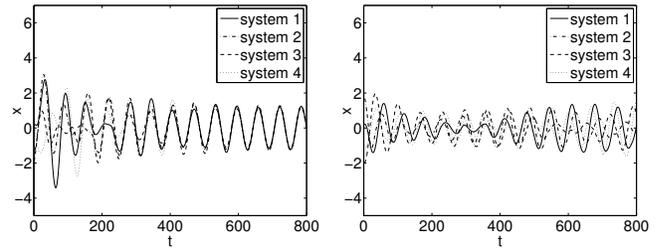
Fig. 2. First component of the solutions of the closed loop harmonic oscillators by using the dynamic control law (to the left) and the static control law (31) (to the right). The dynamic control ensures exponential synchronization. In contrast, synchronization is not observed with the diffusive interconnection.
