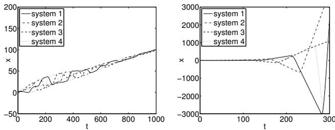
Fig. 3. First component of the solutions of the closed loop double integrators by using the dynamic control law (to the left) and the static control law (34) (to the right). The dynamic control ensures exponential synchronization. In contrast synchronization is not observed with the diffusive interconnection.
