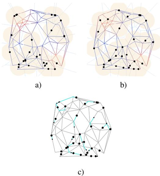
Fig. 2. Deployment problem of 30 sensors in an environment described by a (full) network. Density function  $20 \left( \exp \left( -(x-1)^2 - (y-4)^2 \right) + \exp \left( -(x-4)^2 - (y-1)^2 \right) \right)$ . Figure a) illustrates the initial positions and the Voronoi partition, whereas figure b) illustrates the final positions. Figure c) shows the gradient ascent flow. Notice that sensors are now forced to move on the network.
