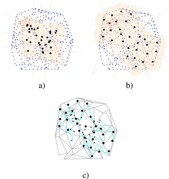
Fig. 1. Deployment problem of 30 sensors in an environment described by a collapsed network. Collapsing factor  $r = 0.3$ , density function  $20 \left( \exp \left( -(x-1)^2 - (y-4)^2 \right) + \exp \left( -(x-4)^2 - (y-1)^2 \right) \right)$ . Figure a) illustrates the initial positions and the Voronoi partition, whereas figure b) illustrates the final positions. Figure c) shows the gradient ascent flow. Notice that sensors can move in  $\mathbb{R}^2$ .
