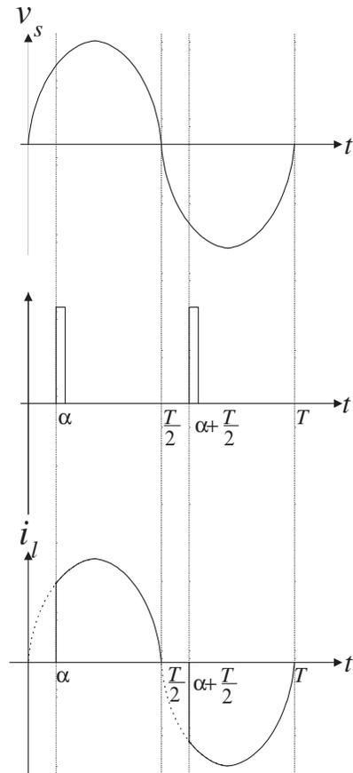
Fig. 4. Waveforms for the semiconverter rectifier.
