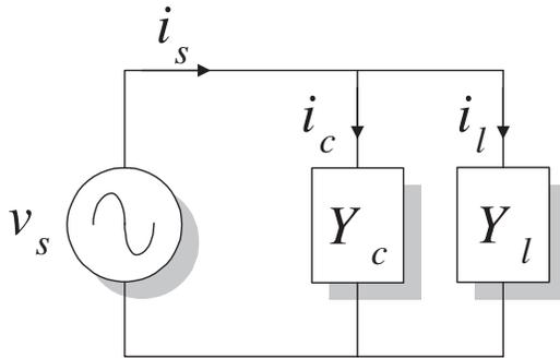
Fig. 2. Circuit schematic of shunt PF compensation configuration.
