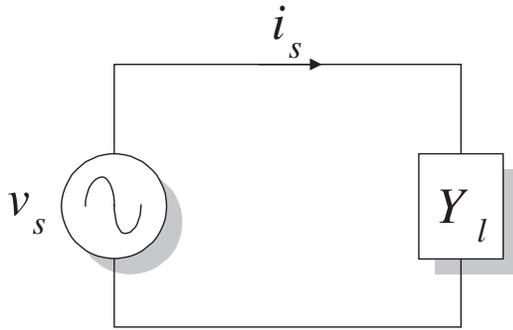
Fig. 1. Circuit schematic of an  $n$ -phase ac generator with negligible impedance connected to a (possibly nonlinear and time varying) load.
