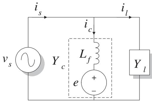
Fig. 6. Circuit schematic of a shunt active filter operating as a PF compensator.
