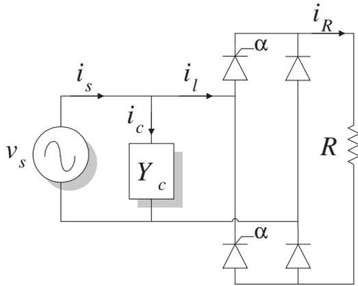
Fig. 3. A semiconverter rectifier load.
