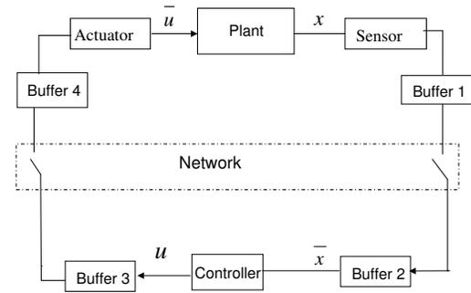
Fig. 1. Structure of a networked control system with packet losses.
