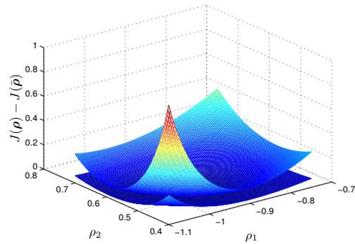
Fig. 3. Surface plot of the normalized performance cost function on a grid for the controller parameters. The lower surface is the performance cost when  $\alpha = 0$  and the upper surface is for  $\alpha = 1$ . The same noise realization  $v_t$  has been used in each grid point and in the perturbation signal design in order to have a smooth surface.
