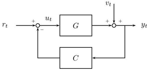
Fig. 2. A general feedback loop designed for disturbance rejection. The process,  $G$ , and the compensator in the feedback loop,  $C$ , is given as scalar linear transfer functions.
