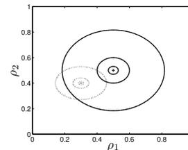
Fig. 1. Contours and minima for two cost functions with equal levels for the contour lines.  $\rho_1$  and  $\rho_2$  are parameter in the controller. The full lines and the cross refer to the original design criterion,  $J_0$ . The dotted lines and the dot in the center is the cost function when affected by an external perturbation,  $J_1$ .
