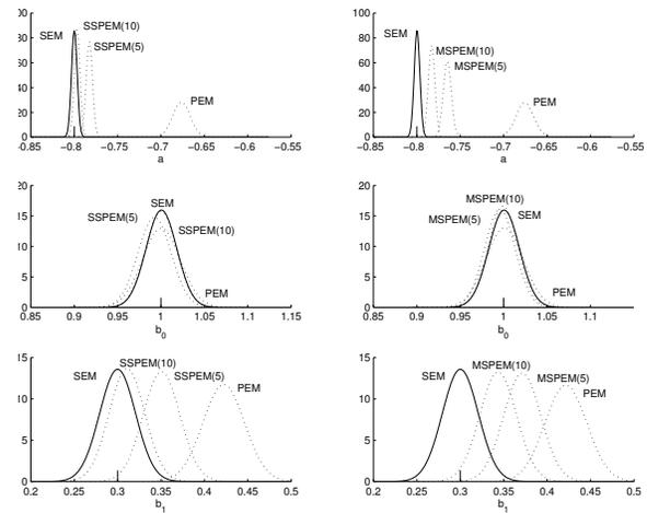
Fig. 4. Probability density functions of the estimates of  $a^o$ ,  $b_0^o$ ,  $b_1^o$  (first, second and third row respectively) obtained by the SEM (solid line), SSPEM (left column, dotted line), MSPEM (right column, dotted line) criteria computed by Monte Carlo simulation in the case of OE noise structure computed for  $k = 1, 5, 10$ , being  $k$  the number of steps ahead.
