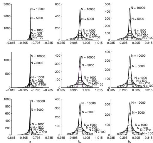
Fig. 2. Probability density functions of the estimates  $a$ ,  $b_0$ ,  $b_1$  (first, second and third column respectively) obtained by the SEM criterion computed by Monte Carlo simulation in the three noise model cases (OE, ARMAX, ARARX, shown in the first, second and third row respectively) computed for different values of  $N$  (100, 250, 500, 1000, 5000, 10000).
