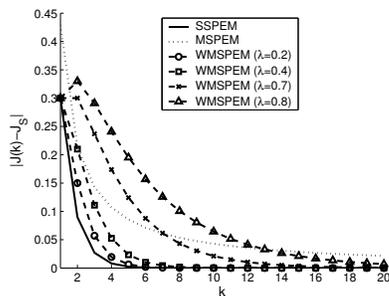
Fig. 1. Bounding functions for the convergence of the SSPEM, MSPEM and WMSPEM ( $\lambda = 0.2, 0.4, 0.7, 0.8$ ) criteria to SEM.
