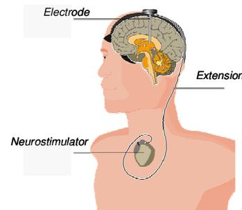
Fig. 1: Schematic of Deep Brain Stimulation System
