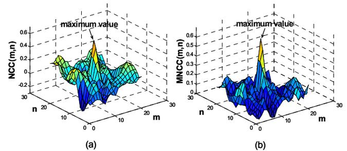
Figure 2: a. Example of normalized cross-correlation map b. Example of multiple normalized cross-correlations map for the same image and template.
