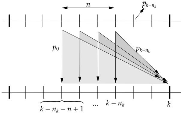
Fig. 8. The Figure illustrates an event where  $n$  consecutive packets arrive before time  $k$ . The packets which arrive may do so at anytime between their transmission time and time  $k$ . The potential arrival times are represented by the shaded area. The sequence of consecutive packets is broken by a packet being delayed with probability  $\bar{p}_{n_k}$ .
