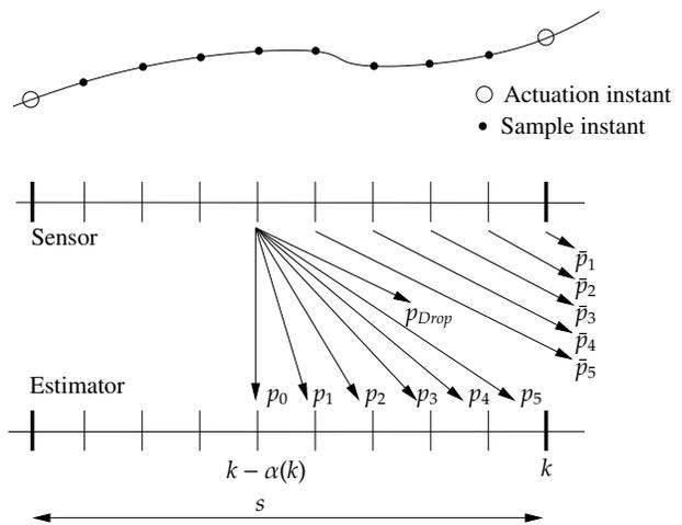
Fig. 3. State observations occur at *sample instants*. Control actions are computed and implemented at *actuation instants*. Actuation instants are separated by  $s$  sample instants. Sensor observations are sent over the network and incur a delay  $i$  with probability  $p_i$ , or are dropped with probability  $p_{Drop} = 1 - \sum_{i=0}^{\infty} p_i$ .
