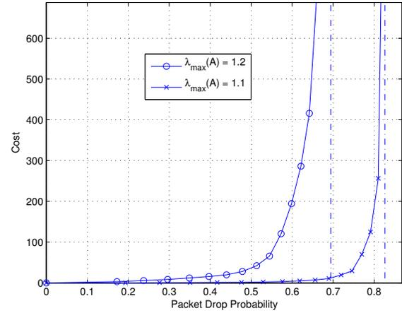
Fig. 7. Each curve represents a different system. Packets are delayed with uniform probability (Figure 4(a)), and dropped when delay exceeds 30. The stability upper bound on  $p_{Drop}$  is indicated by the vertical asymptotes. The upper curve represents a system with a largest eigenvalue of 1.2 and hence a stability bound of  $p_{Drop} = 0.69$ . The lower curve is a system with largest eigenvalue as 1.1 and stability bound of  $p_{Drop} = 0.83$ .
