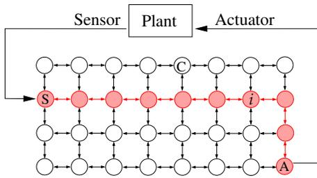
Fig. 1. The controller is at node C, and  $\pi_{SA}^*$  is a minimal path.
