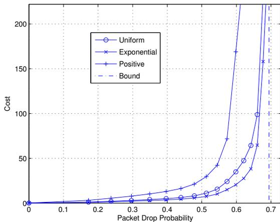
Fig. 6. Packets delayed 30 time steps are dropped. The lowest curve is the cost for exponential packet delay distribution (Figure 4(b)), the middle curve for uniform distribution (Figure 4(a)), and upper curve for linear distribution (Figure 4(c)).
