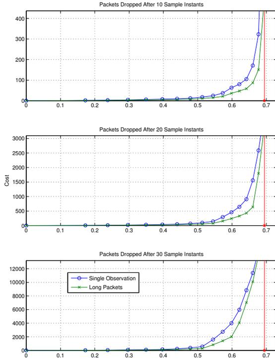
Fig. 5. Packets are delivered with uniform probability of delay as shown in Fig. 4(a). In the top figure, packets delayed by more than 10 sample instants are dropped. In the second and third figures the delay threshold is 20 and 30, respectively. The x-axis is the packet drop probability. The lower curve in each is the cost under LPA, and the upper curve that for system which only transmits a single observation. Notice that the cost diverges at the same packet drop probability in each figure.
