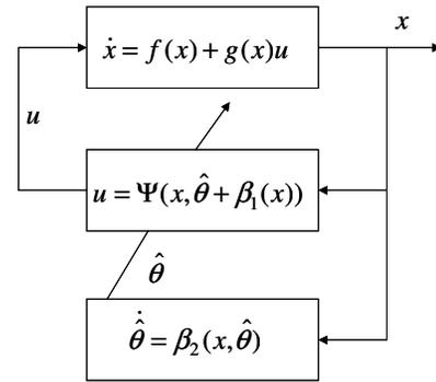
Fig. 1. Continuous-time I&I adaptive control systems
