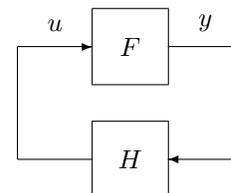
Fig. 1. Feedback system  $\Sigma$  with delay  $H$ .
