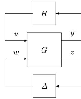
Fig. 2. Uncertain feedback system  $\Sigma_{\Delta}$  with delay  $H$ .
