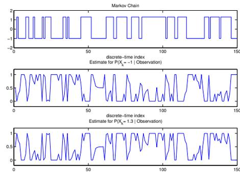
Fig. 1. In this set of three subplots we show the partially observed Markov chain, (2-state), and the estimated (filter) probabilities corresponding to each state.
