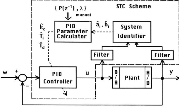
Fig. 2. Block diagram of the temperature control system of a polybutene reactor using the self-tuning PID control scheme.
