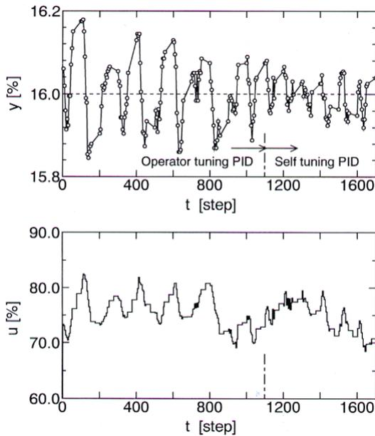
Fig. 4. Control results where the operator tuning parameters were used in the interval  $0 \leq t < 1100$  and the self-tuning PID parameters were used in the interval  $t \geq 1100$ .
