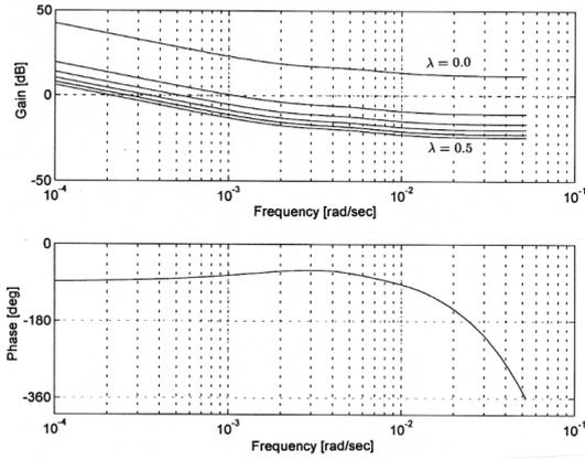
Fig. 3. Bode diagram of the temperature control system of the polybutene reactor to indicate the effect of  $\lambda$ .
