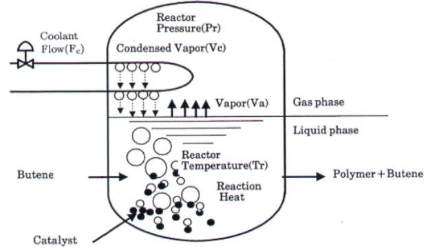
Fig. 1. Schematic diagram of the polybutene reactor.
