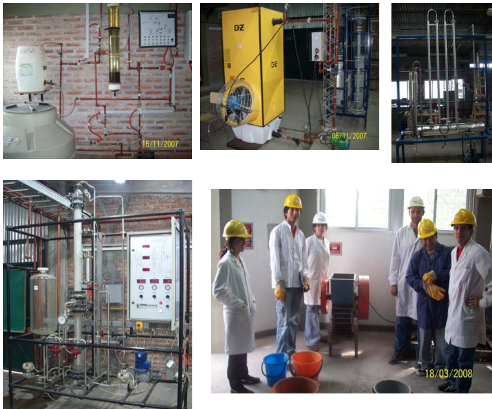
Figure 4 – Pilot Plant II equipment: Softener, Cooling tower, UHT, Absorption tower, Crusher
