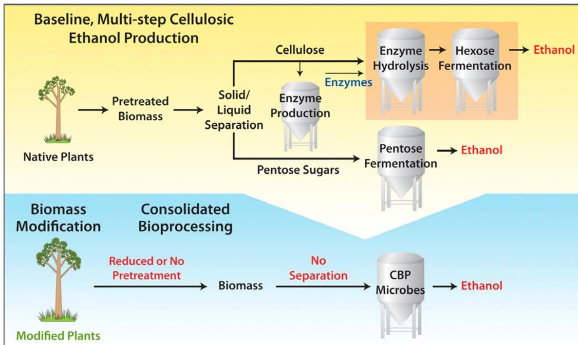
Figure 1: Conceptual baseline for a generation one cellulosic biorefinery.
