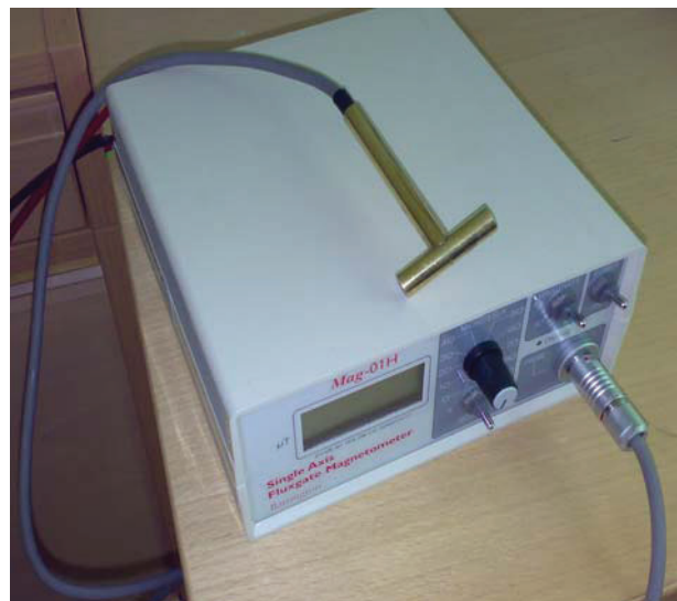
Figure 2 Fluxgate magnetometer Mag-01 (H) and the single-axis probe
