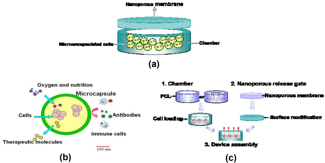
**Figure 1.** Schematic diagram of biodegradable nanoporous membrane systems. (a) integrated device; (b) microcapsule; (c) PCL large capsule with nanoporous gate.
