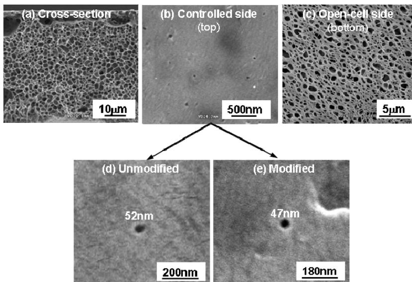
**Figure 2.** SEM images of PCL membrane formed with 20 wt% in mixture of dioxane and 2-Methoxyethanol with a ratio of 15 to 65 by weight (evaporation time: 60 sec, temperature of water bath: 5 °C): (a) cross-section, (b) controlled side from top view, (c) open-cell side from top view, (d) controlled side of unmodified PCL membrane using higher magnification, and (e) controlled side after PEG grafting.
