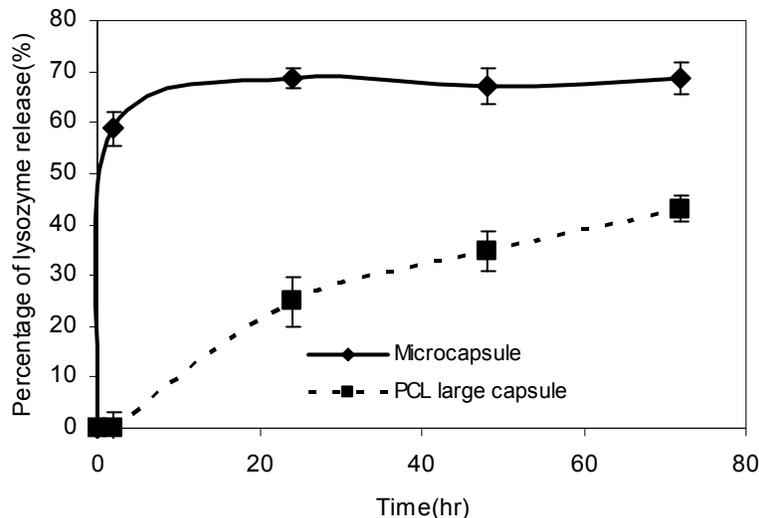
**Figure 3.** Lysozyme diffusion through the nanoporous membrane in microcapsule and PCL large capsule systems.
