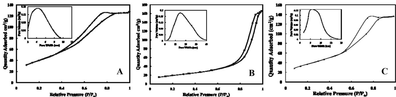
**Figure 2.** Nitrogen adsorption-desorption isotherms and pore size distribution of mesoporous  $\text{Ga}_2\text{O}_3$  phases synthesized using (A) F127, (B) P123, (C) CTAB.
