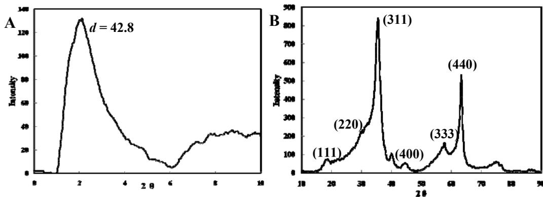
**Figure 3.** (A, B) X-ray diffraction pattern of the mesostructured Gallia synthesized using triblock copolymer, indicating a cubic spinel-type structure.
