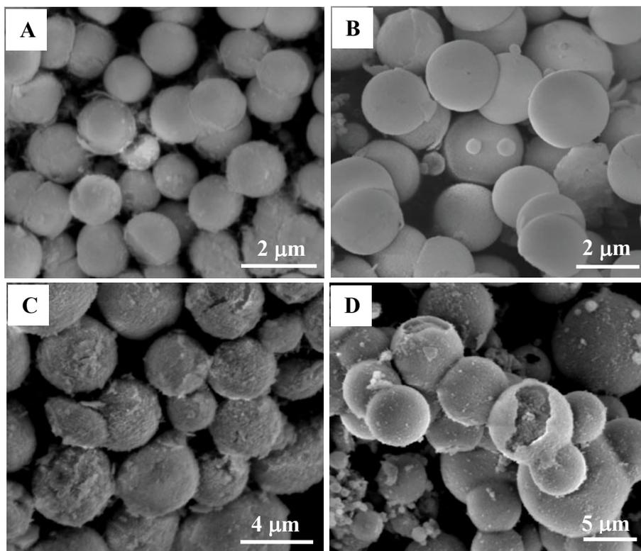
**Figure 1.** SEM images of mesoporous  $\text{Ga}_2\text{O}_3$  phases with increasing size of the crystals with respect to the Hydrothermal Temperature (A)  $1.8 \mu\text{m}$  at  $150^\circ\text{C}$ , (B)  $2.2 \mu\text{m}$  at  $180^\circ\text{C}$ , (C)  $4.5 \mu\text{m}$ , and (D)  $6.5 \mu\text{m}$  at  $200^\circ\text{C}$ .
