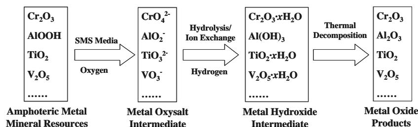
Fig. 10. Target Element Conversion Process for the SMS Platform
