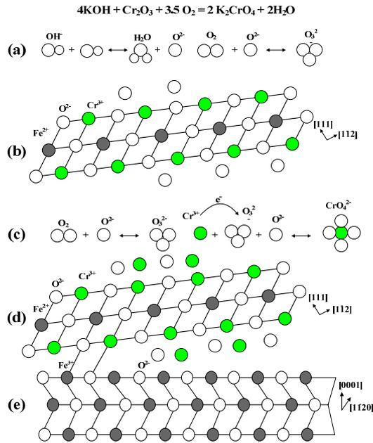
(a) dissolution of oxygen and creation of oxygen anion; (b) main body of chromite ore particle and  $\text{FeO}\cdot\text{Cr}_2\text{O}_3$  crystal; (c) oxidation of trivalent chromium ion; (d)  $\text{FeO}\cdot\text{Cr}_2\text{O}_3$  crystal structure destroy,  $\text{Cr}^{3+}$  dissociation, and product dissociation; (e) creation of  $\text{Fe}_2\text{O}_3$  product layer.
