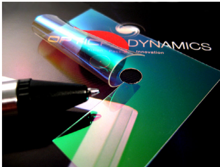
Figure 2: A 9-layer nanocomposite thin-film coating on a polymer substrate demonstrating high flexibility and transparency.
