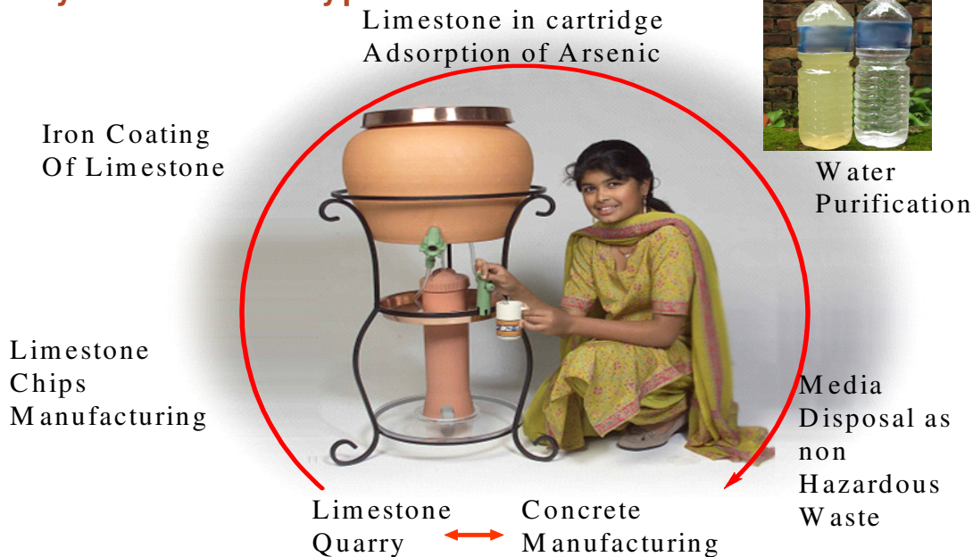
Figure 4: Sustainable Process using Iron Coated Limestone.
