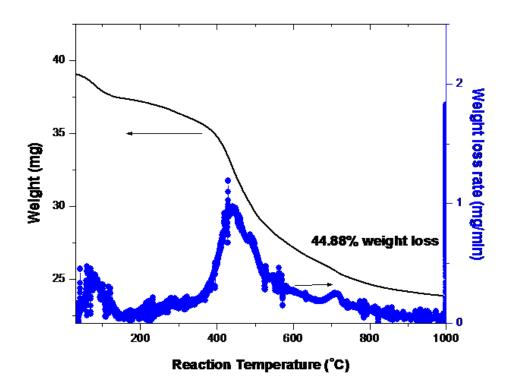
Additional weight loss of 55% due to combustion reaction was observed when air was introduced at  $1000\,^{\circ}$ C subsequent to the  $N_2$  introduction. When coal was heated in  $CO_2$  the weight loss profile and rate data were similar to that with  $N_2$ . This indicated that the presence of  $CO_2$  did not have any significant effect on the process.
