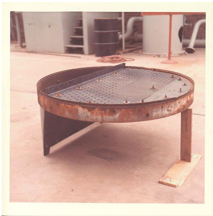
Figure 1. 14% Hole Area Commercial Sieve Tray
