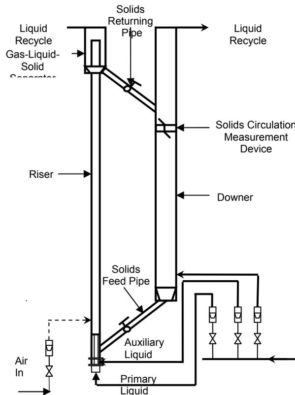
Figure 1: Schematic Diagram of GLSCFB system
