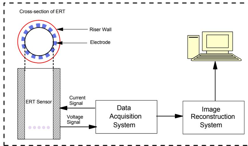
Figure 2: Schematic diagram of the measurement principle of ERT.
