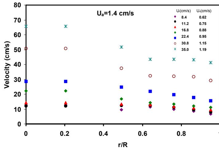
Figure 6: Radial distribution of combined gas-solid phase propagation velocity profile under different superficial liquid and solid velocities for glass beads.
