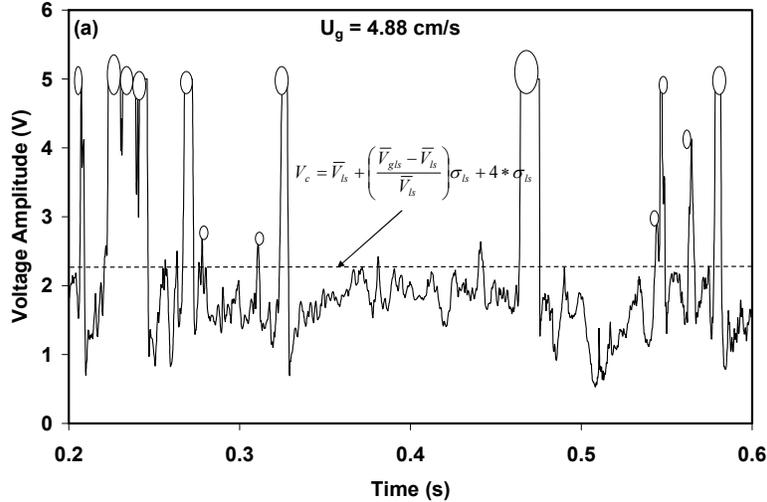
Figure 4: Gas holdup measurement method using optical probe.
