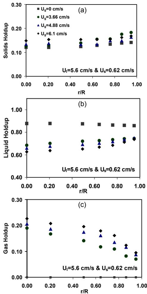
Figure 5: Radial distribution of (a) solids (b) liquid and (c) Gas phase holdups under different gas superficial velocity at  $U_l = 5.6 \text{ cm/s}$  &  $U_s = 0.62 \text{ cm/s}$  using glass beads.
