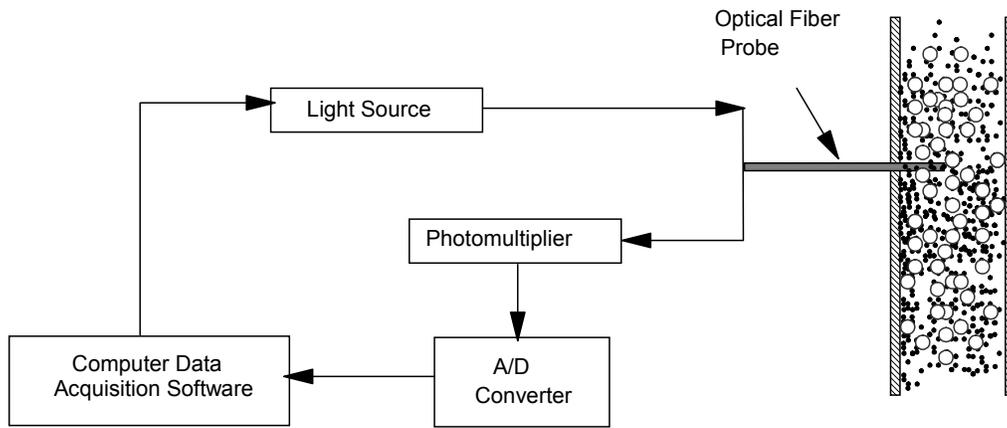
Figure 3: Optical Fibre Probe system for gas holdup measurement in GLSCFB riser.
