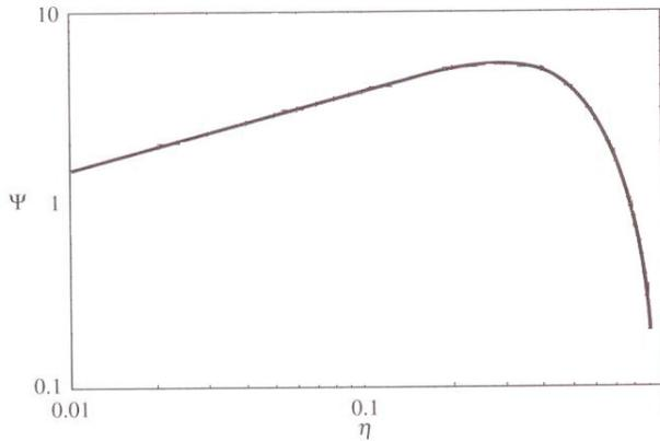
Figure 2.- Effect of a lubricant layer on the flow through a tube.
