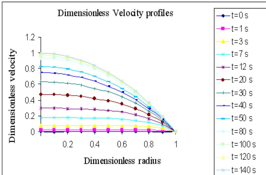
Figure 3.- Dimensionless radial velocity profiles at different times.
