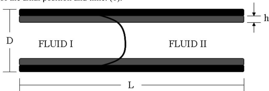
Figure 1. - Laminar flow of fluid I through a lubricated tube. Flow II is the lubricant with constant thickness h (1).
