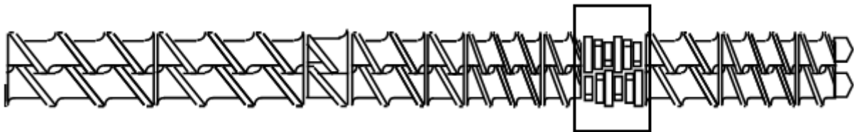
Fig 1. Example screw design with the highlighted section indicating the variable zone.
