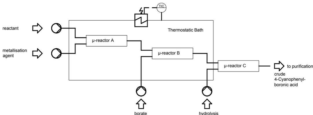
**Figure 1.** Simplified flow sheet of the reaction plant
