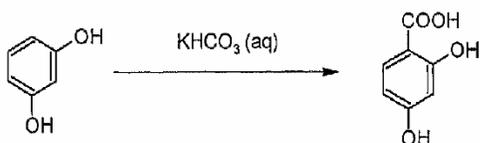
The investigated process here is the aqueous Kolbe-Schmitt synthesis of 2,4-dihydroxy benzoic acid from resorcinol in an aqueous solution of potassium hydrogen carbonate under high temperature of 200 °C and high pressure of 40 bar in a continuous working microreaction plant (Fig. 5). The reaction times could be reduced by three orders of magnitude, from some hours for the batch process to some tens of seconds. The achieved selectivity was 45 % [24].
