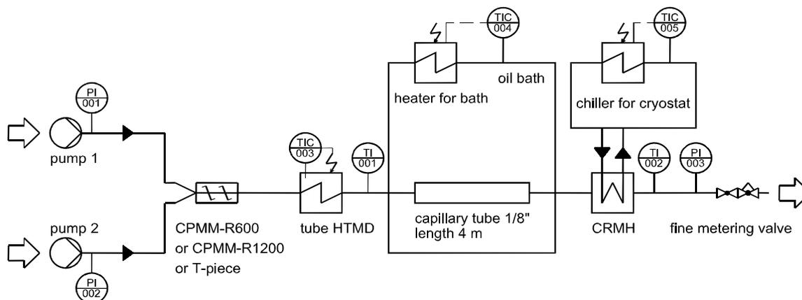
**Figure 5.** Flow sheet of the reaction plant
