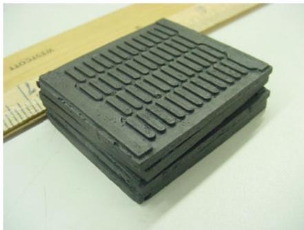
**PIP test plate stack to be laminated**
