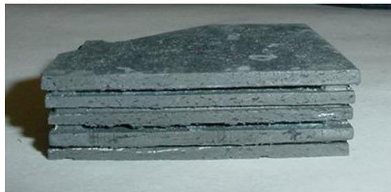
**PIP test plate stack after lamination and pyrolyzation processes**
