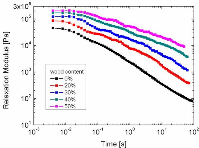
**Figure 5.** Relaxation Modulus of HDPE-Wood Composites.
