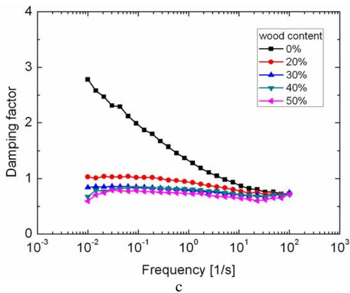
**Figure 2.** Storage Modulus (a), Loss Modulus (b) and Damping Factor (c) of HDPE-Wood Composites.
