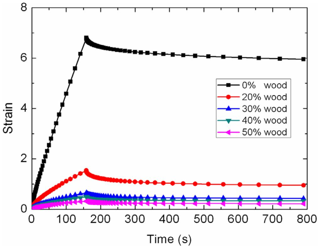
Figure 4. Strain Response of HDPE-Wood Composites.
