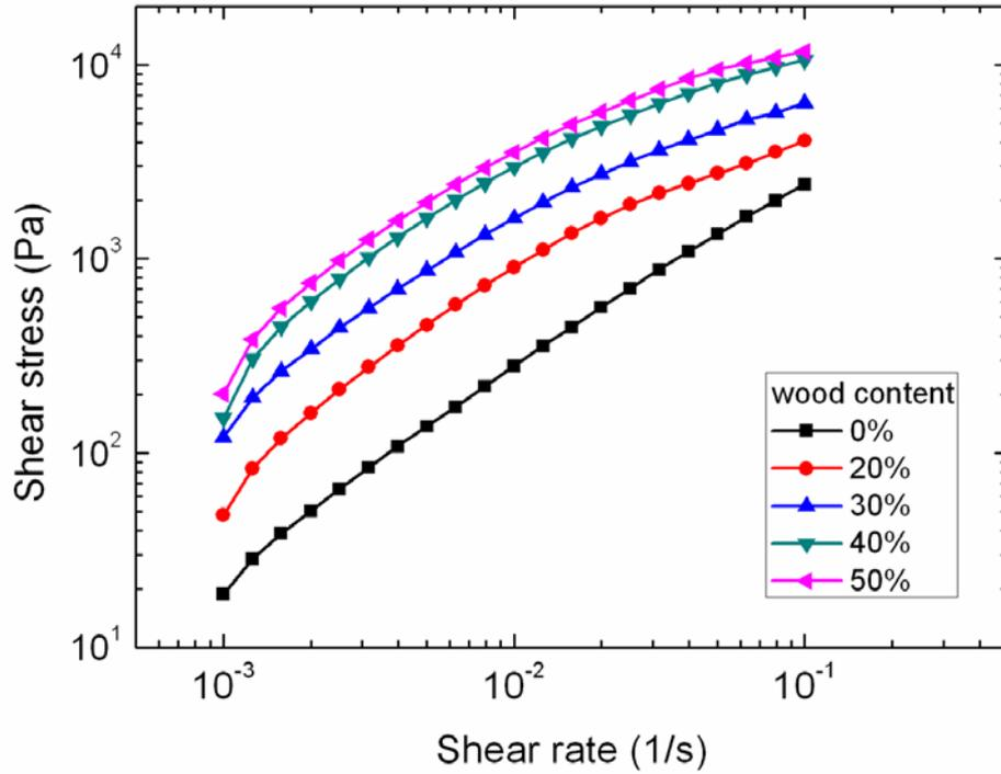
**Figure 1.** Steady Shear Sweep Data of HDPE-Wood Composites.
