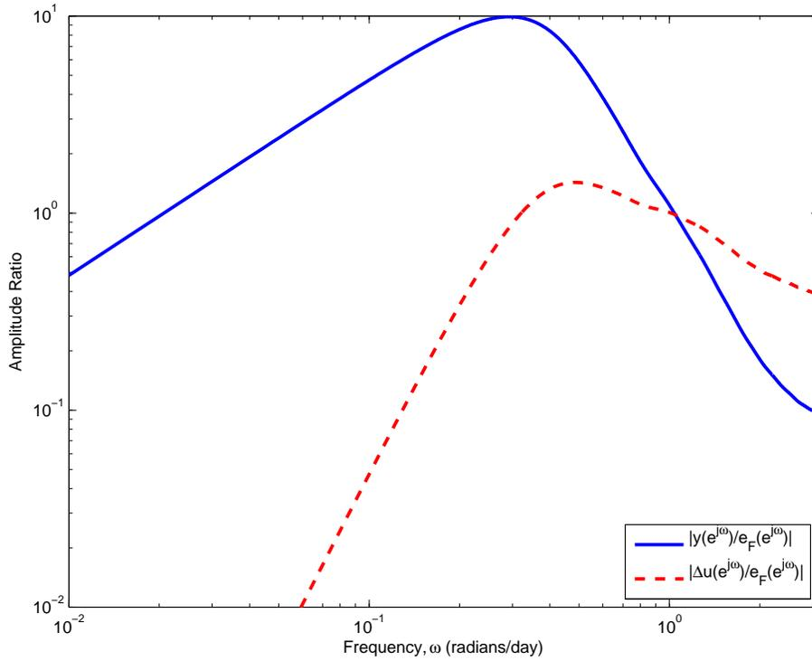
Figure 5: Amplitude ratio of the inventory and starts change response to forecast error ( $\frac{y(e^{j\omega})}{e_F(e^{j\omega})}$  and  $\frac{\Delta u(e^{j\omega})}{e_F(e^{j\omega})}$ , respectively) for the model and controller parameters per Fig. 4.
