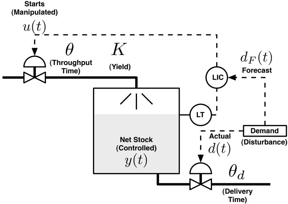
Figure 1: Fluid analogy: a single manufacturing node represented as a system of pipes and a tank.
