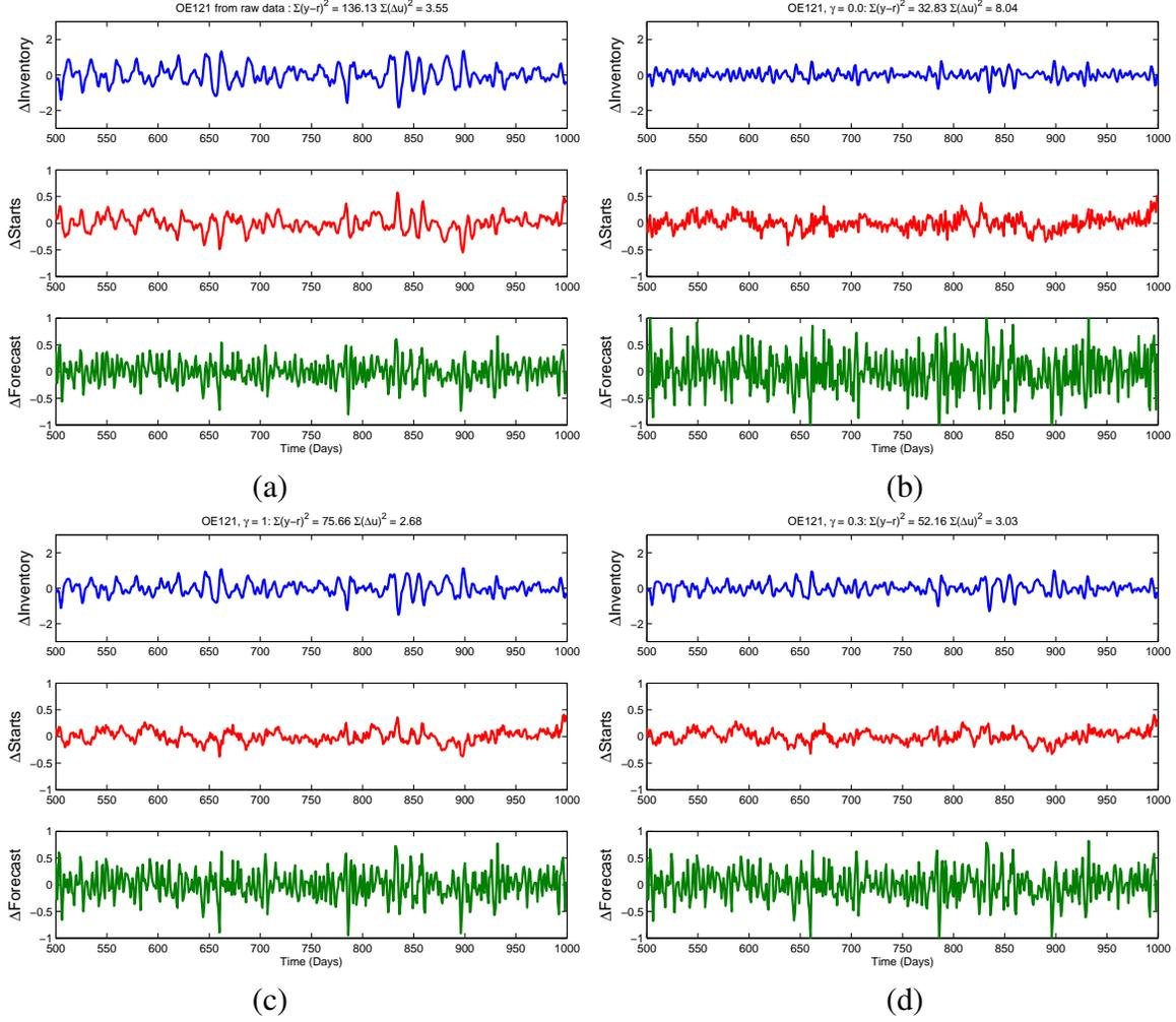
Figure 7: Time series for closed-loop responses of the production/inventory system where the demand forecast is developed from (a) an OE-[1 2 1] fit to unfiltered data, (b) an OE-[1 2 1] fit to control-relevant filtered data ( $\gamma = 0.0$ ), (c) an OE-[1 2 1] fit to control-relevant filtered data ( $\gamma = 1.0$ ), and (d) an OE-[1 2 1] fit to control-relevant filtered data ( $\gamma = 0.3$ ).
