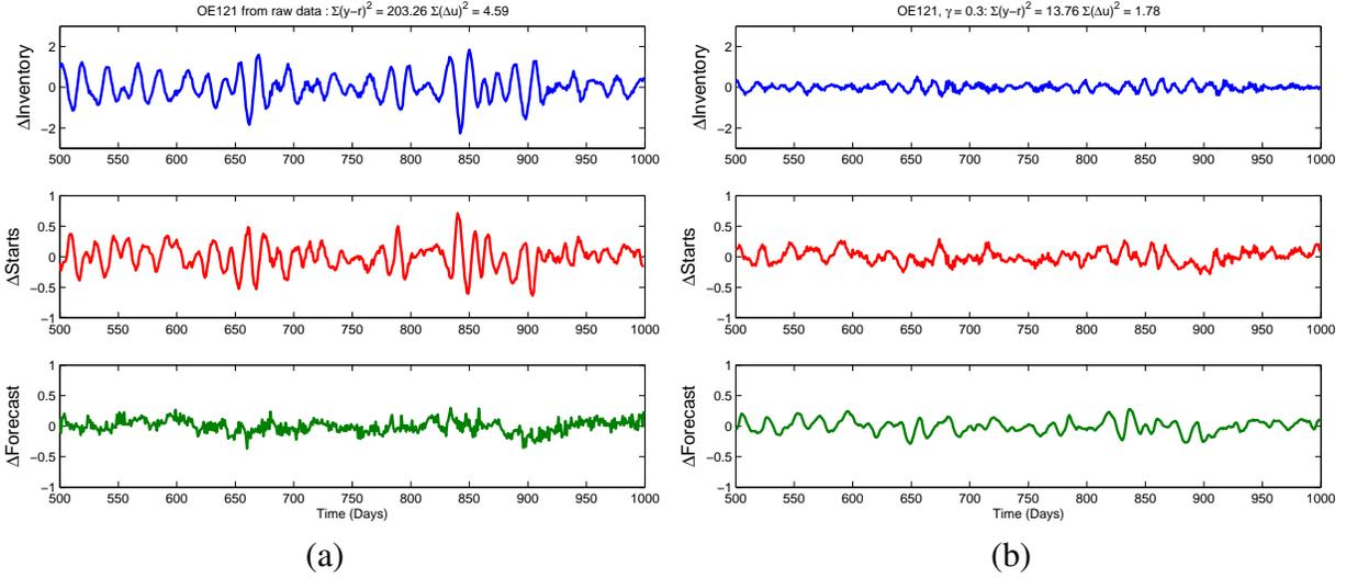
Figure 10: Time series where the demand forecast is developed from (a) an OE-[1 2 1] fit to unfiltered data ( $\Sigma(y - r)^2 = 203$ ,  $\Sigma(\Delta u)^2 = 5$ ) and (b) an OE-[1 2 1] fit to control-relevant filtered data ( $\Sigma(y - r)^2 = 14$ ,  $\Sigma(\Delta u)^2 = 2$ ) obtained from the user defined weighting function ( $\gamma = 0.3$ ).
