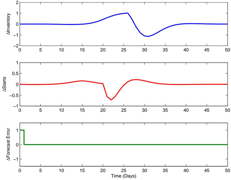
Figure 4: Supply chain control system response to a unit forecast error pulse. Throughput time:  $\theta = 5$  days, prediction horizon:  $p$  and  $\theta_F = 20$  days, move horizon:  $m = 10$  days, move suppression:  $Q_{\Delta u} = 5$ , control error weight:  $Q_e = 1$ .
