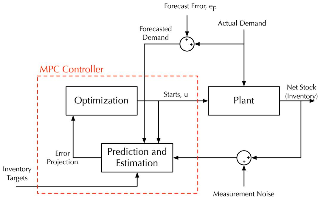
Figure 3: Block diagram schematic of Model Predictive Control, highlighting the introduction of forecast error,  $e_F$ .
