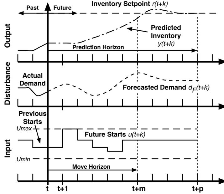
Figure 2: Receding horizon representation of Model Predictive Control.
