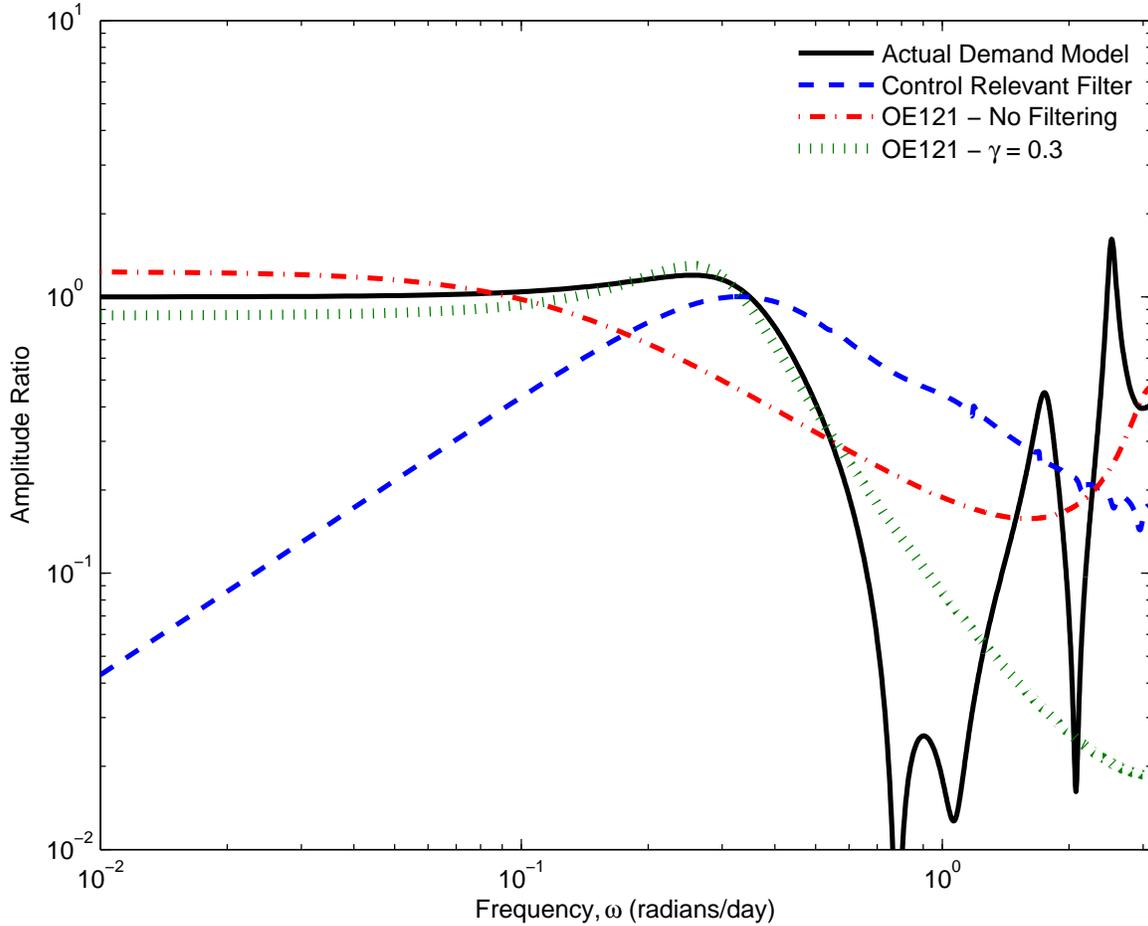
Figure 9: Corresponding frequency responses where the demand forecast is developed from an OE-[1 2 1] fit to unfiltered data and an OE-[1 2 1] fit to control-relevant filtered data obtained from the user defined weighting function ( $\gamma = 0.3$ ).
