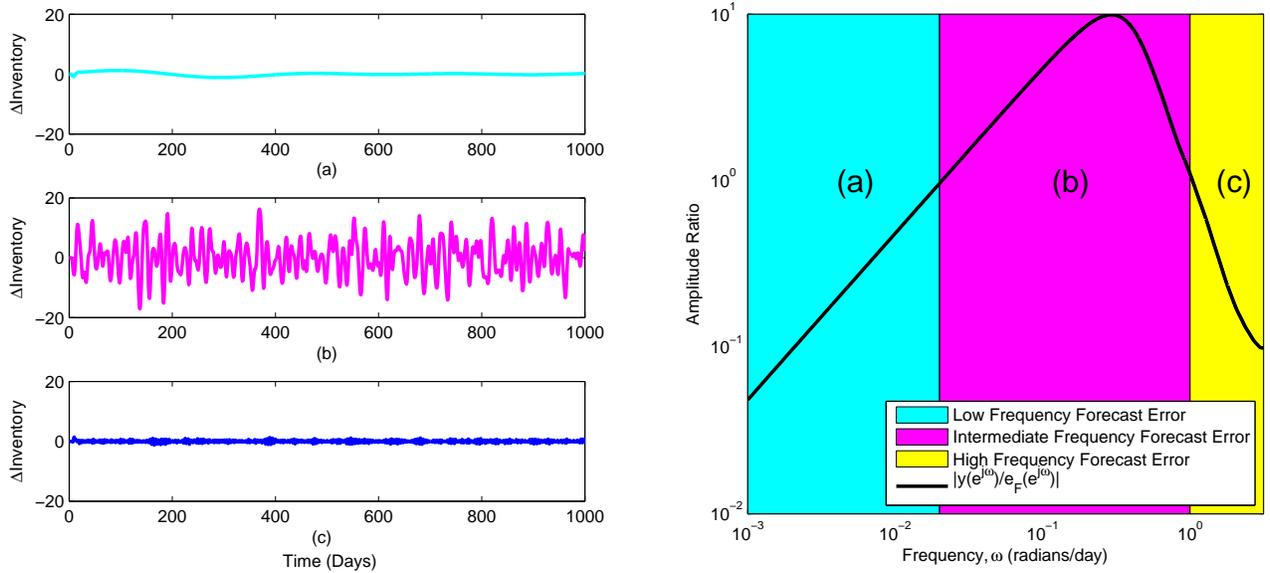
Figure 6: Inventory response of the closed-loop production/inventory system to low frequency (a), intermediate frequency (b), and high frequency forecast error (c).
